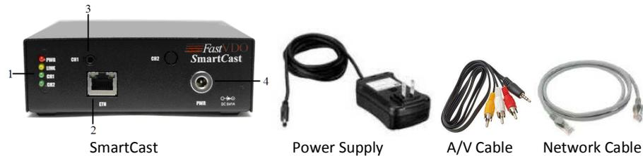
1. Status LED    2. Ethernet port    3. Ch-1 A/V input    4. Power supply input
